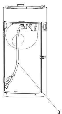
Connect the hose and regulator. See *Connecting the gas bottle*
