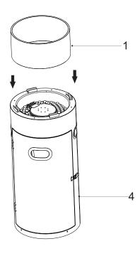
Place the protective glass ring over the burner. NEVER use the device without protective glass.
